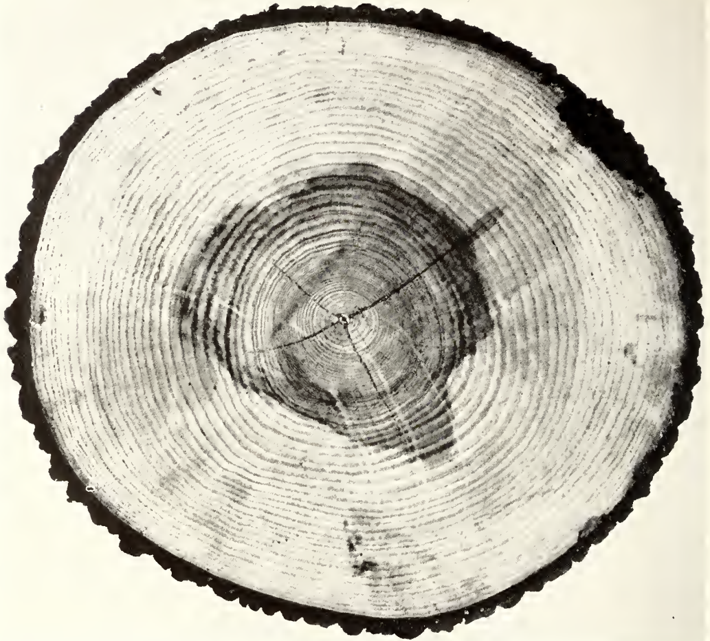
FIGURE 2-1.—Cross section of white ash log, showing irregularly shaped heartwood at center, wide sapwood, annual rings in both sapwood and heartwood, and bark.
